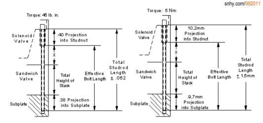
To simplify the installation of ISO 03 and ISO 05 sandwiches, Sun offers uncut (can be cut to length in the field) or precut studkits in both inch and metric standard threaded rod. Once the rods are installed in a subplate or manifold, they act as a guide in assembling the sandwich body stack. After the directional control valve is assembled on top of the stack, Sun studnuts are used to retain the assembled stack.
